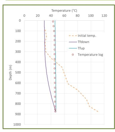
Comparison between experimental data (red dots) and GEOPIPE model forecast (blue line)
