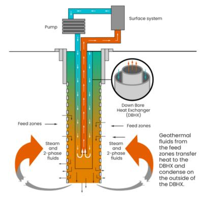
Condensed geothermal fluids descend to the bottom of the DBHX and recirculate back to the reservoir.
