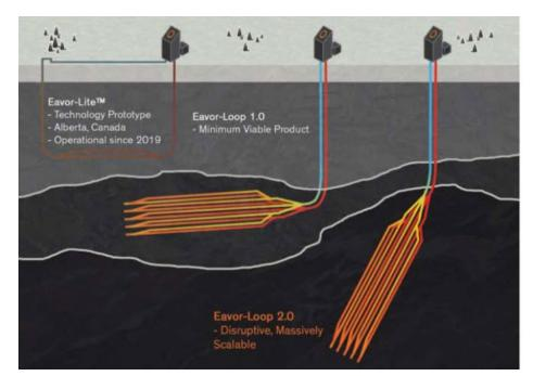
Closed-loop geothermal is an encapsulated system within which a proprietary working fluid is contained and circulated to harvest heat from deep in the earth to be used for commercial heating applications (ex: greenhouses or district heating) or to be used to generate electricity using conventional heat to power engines.
